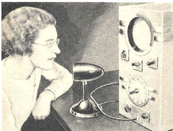
By singing into the microphone attached to this electronic resonoscope device, this singer can determine whether her voice is properly pitched. A cathode-ray tube provides visual images of wave forms of musical notes under observation.
