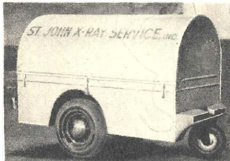
The body of this special three-wheeled trailer contains a compact X-ray apparatus that is used to examine welds in bridge and building construction. Ray pierces three-inch steel.
