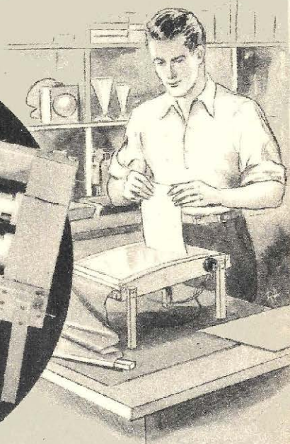
This illustration shows the print dryer in use. The squeeze plate is laid on the top of the dryer, face up, with the prints in position. A cloth band draws prints down flat.
