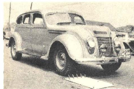
When the tires of this auto are punctured they merely drop about one inch and ride on a specially constructed tube set within the inner tube, enabling driver to make safe stop.
