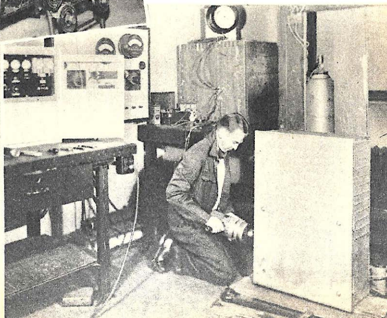
The mechanical robot which produces six motions of the human hand for endurance tests of electrical switches. If the switches stand up under this test, they are approved.
